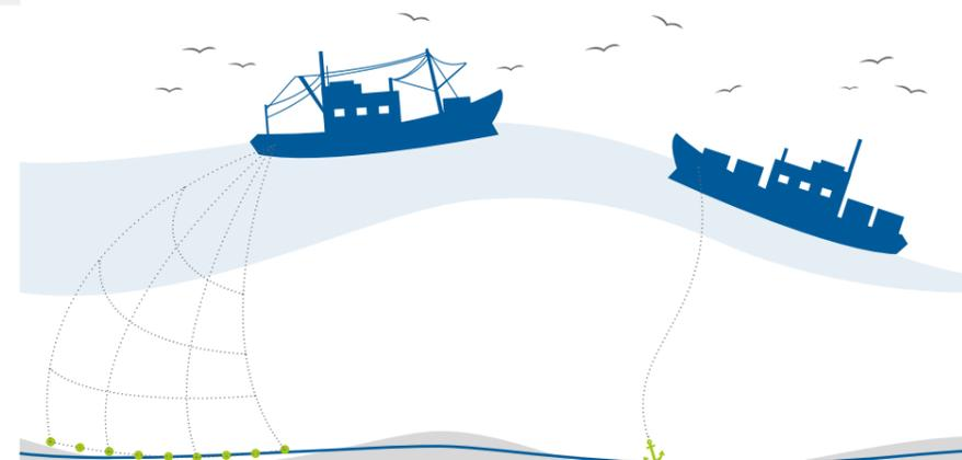
The biggest threats to submarine cables: External forces exerted by heavy ships' anchors and trawl nets of fishing boats at all sea depths.
